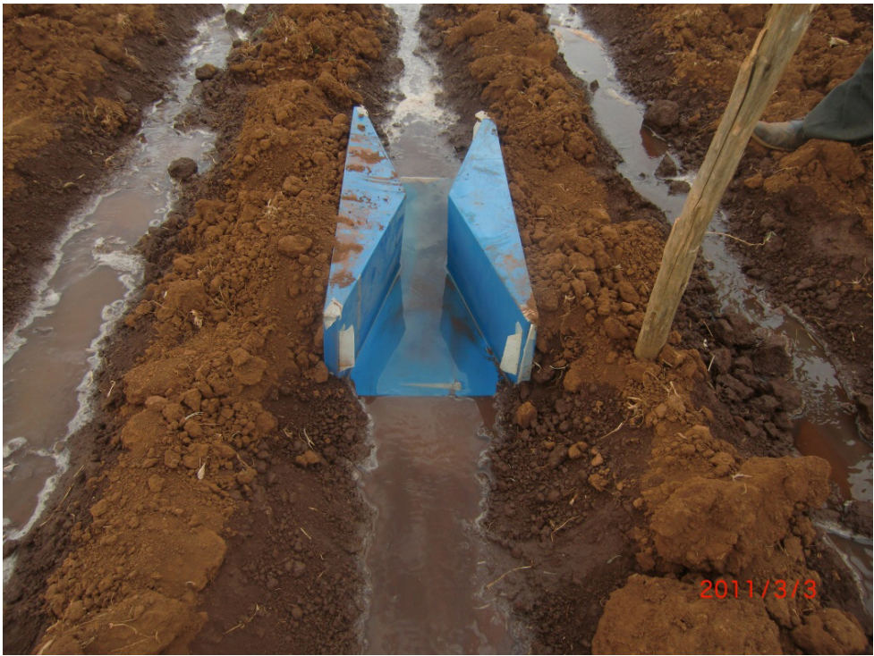
Figure 3.5: Cutthroat flume operation at Koga irrigation field
