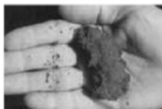
Figure 2.15: feel method of monitoring soil moisture
