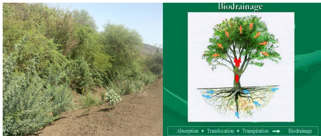
Figure 5.7: principle of bio-drainage and Worer research center experimental field
