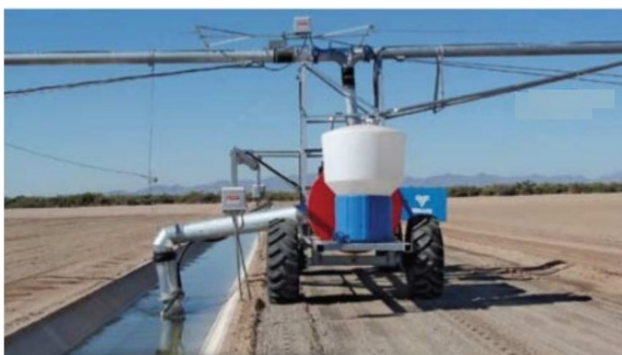
Figure 1-4: Linear move system directly pumping water from canal
