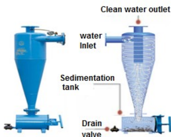
Figure 1-9: Hydrocyclone filter
