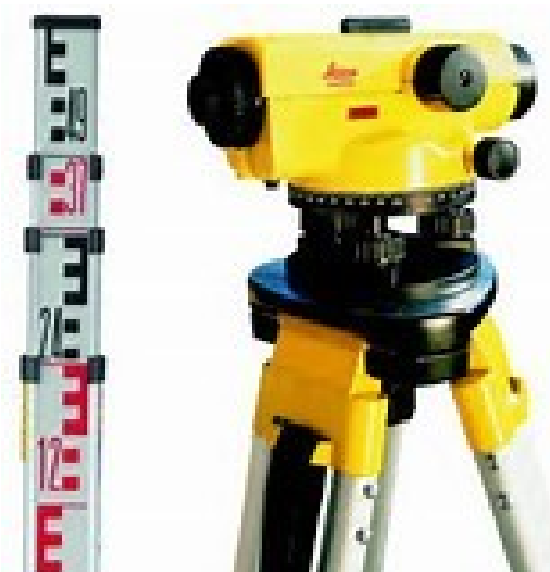
Figure 3-3: Engineer's levelling device (L) and staff (R)
