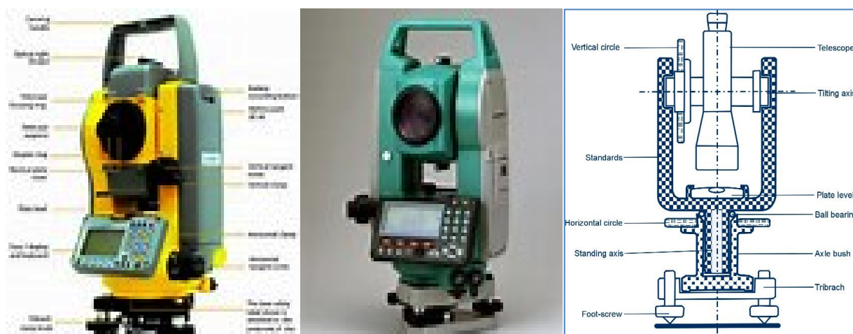
Figure 3-2: Essential features of leica total station (L) & theodolite (R)
