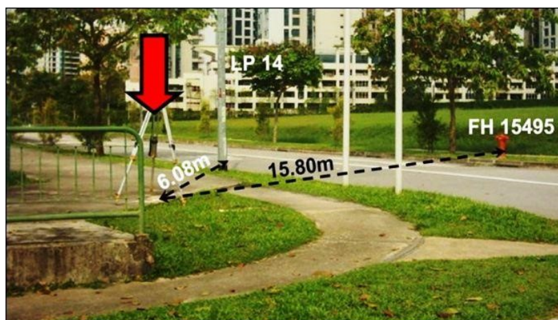
Figure 5-5: Typical digital photograph of control points (GPS station location)
