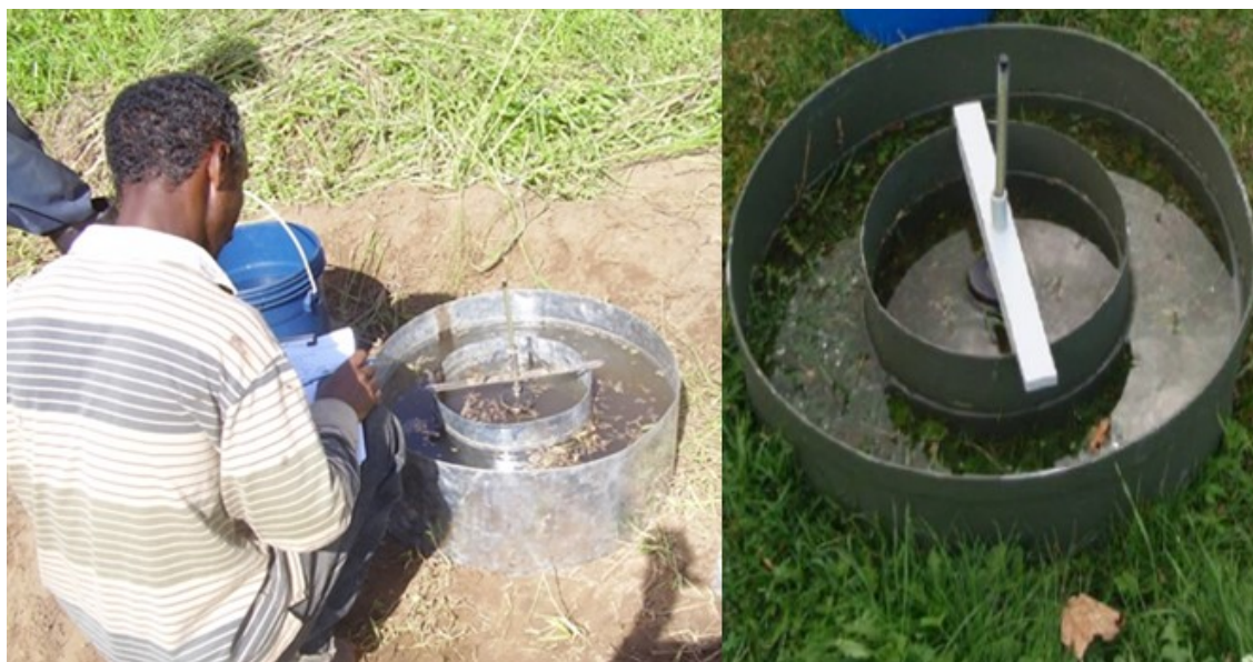
Figure 4-7: Double ring infiltrometer
