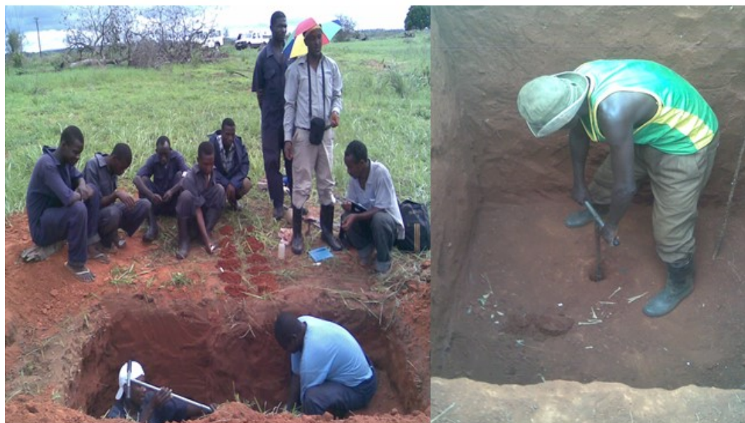
Figure 4-5: Deep boring at the base of profile below 200cm
