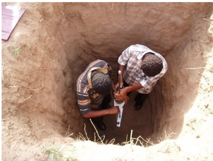
Figure 2-4: Assembling the dynamic cone penetrometer inside test pit to conduct the test, TR-39
