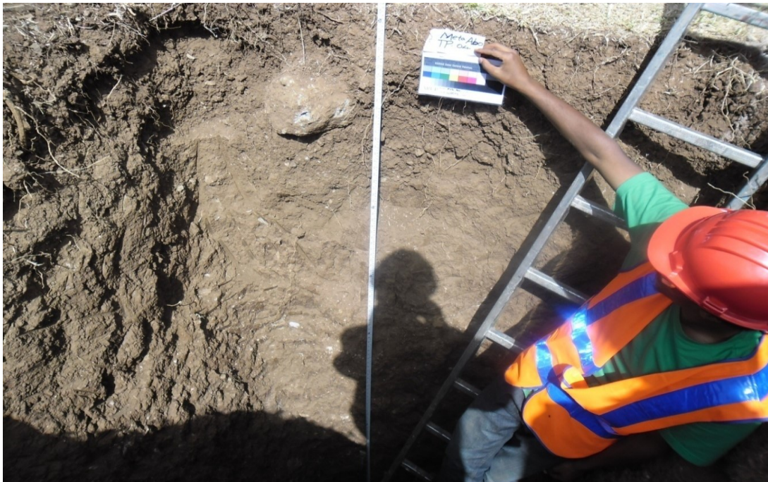
Figure 2-1: Excavated test pit on logging and describing
