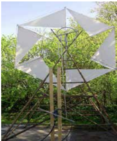
Figure 92: Windmill for Water Abstraction Prototype
