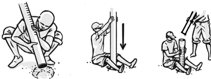
Figure 72: Installation of PVC Casing
