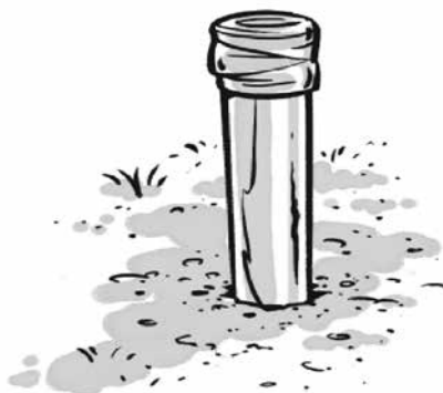
Figure 75: Covering PVC Casing
