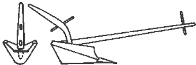
Figure 114: Ridger Plough: (a) Wooden Body, Animal-Drawn
