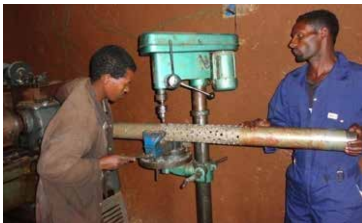
Figure 49: Preparation of Perforated Screen at Local
